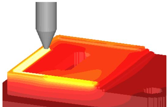
*AdditiveLab DED process simulation predicting temperature profiles of the part to be produced.*
