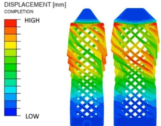
*Simulation of Spinal Cage showing the Displacement distribution via AdditiveLab mechanical analysis; left: lateral view, right: frontal view.*
