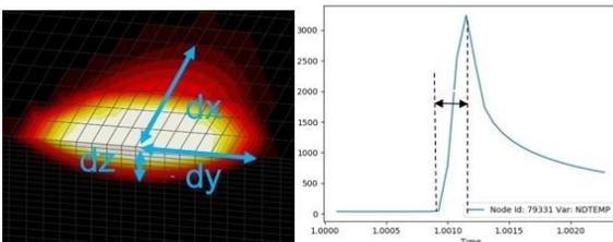
*The temperatures in a cross section cut to measure the melt pool dimensions (left) and the temperature vs. time plot queried at the center of the simulation model.*
