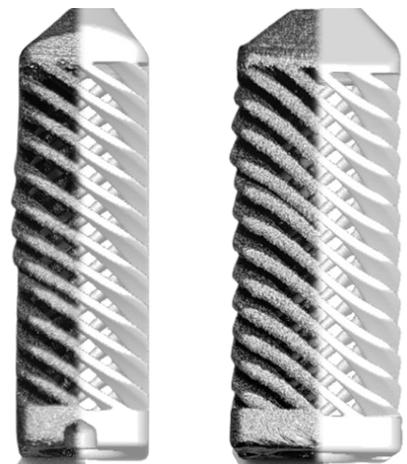
*Production result of Counter-Deformed Spinal Cage showing the Displacement distribution; left: lateral view, right: frontal view mapped against original part design (Courtesy of Tangible Solutions).*
