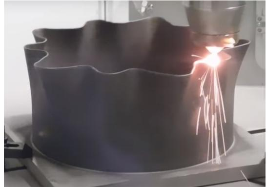
*AM machine printing a part via DED process. (Ref BeAM machines, [www.beam-machines.com](http://www.beam-machines.com)).*
