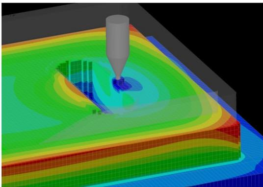
*AdditiveLab DED process simulation predicting displacement zones of the part to be produced.*
