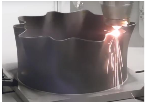
AM machine printing a part via DED process. (Ref BeAM machines, www.beam-machines.com ).
